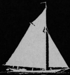
SLOOP — A small to medium-sized fore-and-aft-rigged one-master. This is a Hudson River sloop; sloops in the coastal trade usually had smaller sail plans.
