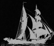
HERMAPHRODITE BRIG — A two-masted vessel whose foremast is square-rigged and whose mainmast is fore-and-aft-rigged.
